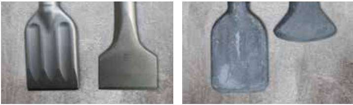
Before use After 10 hours Enduro Standard Enduro Standard
